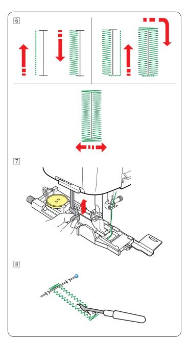
6 The buttonhole is sewn automatically in the sequence shown. When the buttonhole is finished, the machine will stop automatically with the needle in the up position. Press the thread cutter button and remove the fabric.
