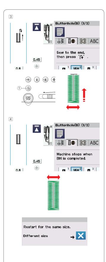
3 Start sewing again, and the machine sews the front bartack and right side of the buttonhole.
