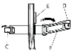
3. Close the holding plate (D) and secure the end with the clasp (C). Make sure that the elastic is in the groove (F). Slide the slide plate (H) with your finger so that the holding plate guides the left side of the elastic tape.
