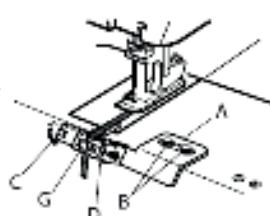
4. Place the fabric under the presser foot, and sew together with the elastic. (Test stitching before sewing actual fabric.)
