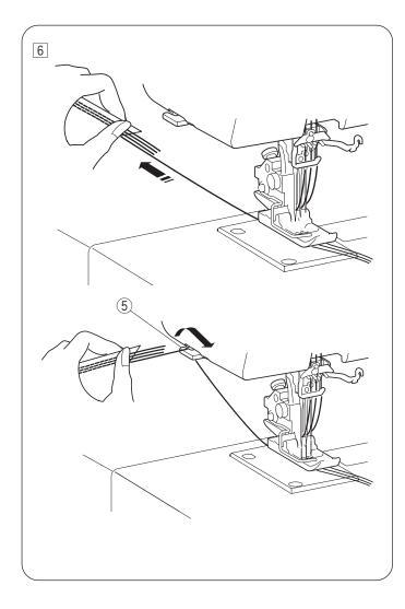
6 Hold the seam tightly and pull the fabric to the rear, then cut the looper thread with the thread cutter.
