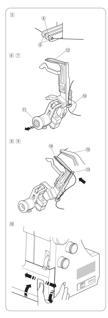
5 Turn the handwheel toward you several times to align the eye of the looper take-up lever and both guide holes.
