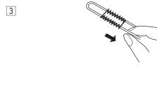
3 Pull the loose ends of the filler cord to tighten it.
