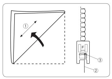
Use a lightweight fabric (tricot, for example). Fold the fabric in bias as shown and stitch on the fold.
