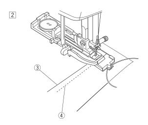
2 Start the machine and sew the buttonhole. Each side of the buttonhole and the bartacks will be sewn over the cord.
