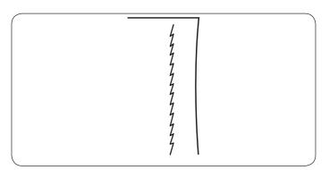
This stitch is a narrow stretch stitch designed to eliminate puckering on knit fabrics and bias seams, while permitting the seam to be pressed completely open flat. Use this stitch for seaming fine fabrics.
