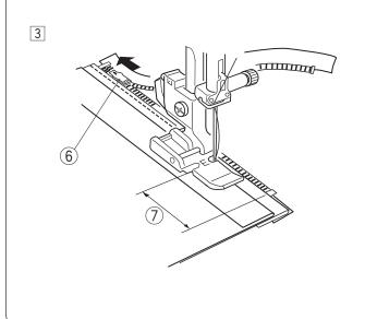
3 Sew through all layers next to the fold. Stop the machine 5 cm (2") before the foot reaches the slider on the zipper tape. Lower the needle slightly into the fabric.
