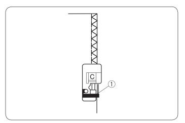
This stitch is used to seam and overcast fabric edges at
