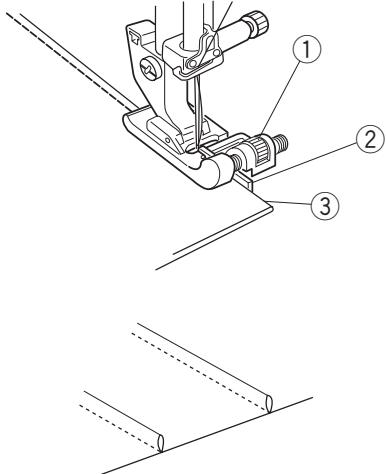
Fold a fabric wrong side together and Lower the needle into the fabric 0.1 – 0.2 cm inside the folded edge.
