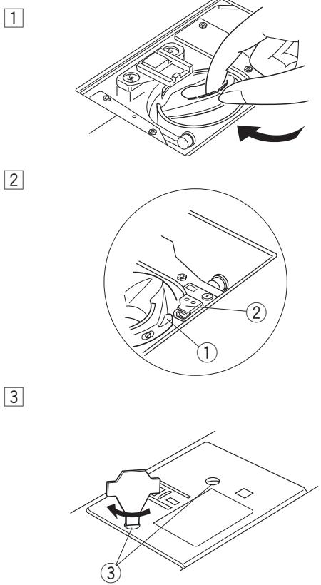
① Insert the bobbin holder into the hook race.
