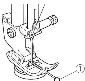
A pin can be placed on the foot to form a shank. Make sure to check if the needle enters into both holes in the button.
