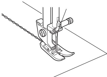
The pattern is sewn with two stitches forward and one stitch backward, forming a seam that does not rip easily.
